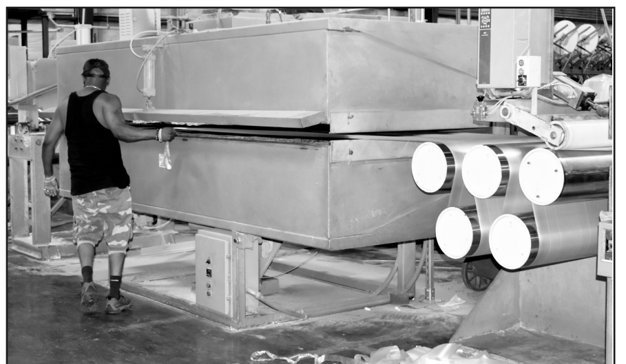
Above, in the left photo, Shop Steward Anthony James works near a machine used to create and spool Poly-Fill, commonly used to fill cables. In right photo, shop steward Anthony James pulls polypropylene film through a machine, an early step in the process of creating Poly-Fill.
