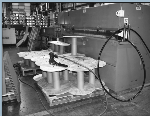
These machines are used to "run a tether," which is the process of putting a jacket over the yarns coming off the wall (seen in the image on the right) to make a tether which is used by the Department of Homeland Security. This particular machine (left) has a runtime of up to 8 hours and produces 23,500 feet of cable.
