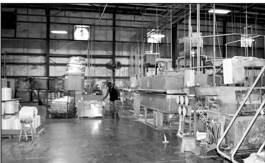
Above, in the left photo, Shop Steward Anthony James works near a machine used to create and spool Poly-Fill, commonly used to fill cables. In right photo, shop steward Anthony James pulls polypropylene film through a machine, an early step in the process of creating Poly-Fill.
