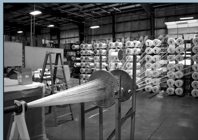
These machines are used to "run a tether," which is the process of putting a jacket over the yarns coming off the wall (seen in the image on the right) to make a tether which is used by the Department of Homeland Security. This particular machine (left) has a runtime of up to 8 hours and produces 23,500 feet of cable.
